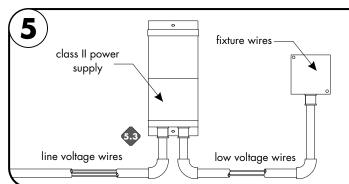
5.1 Ensure the correct (wattage & voltage) power supply is used to power the fixture. Then proceed to connect the fixture wires from fixture to the power supply. For more information please refer to power supply wiring instructions.
